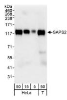
**Detection of human SAPS2 by western blot.** *Samples:* Whole cell lysate from HeLa (5, 15, and 50 µg) and HEK293T (T; 50 µg) cells. *Antibody:* Affinity purified rabbit anti-SAPS2 antibody A300-970A-T used at 1:1000. *Detection:* Chemiluminescence with an exposure time of 3 seconds.
