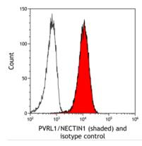
Detection of human PVRL1/NECTIN1 (shaded) in FaDu cells by flow cytometry. *Antibody:* Rabbit anti-PVRL1/NECTIN1 recombinant monoclonal antibody [BLR274L] (A700-274) or isotype control (unshaded). *Secondary:* DyLight® 650-conjugated goat anti-rabbit IgG (A120-101D5).
