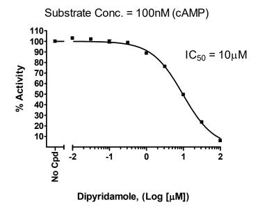
Inhibition of PDE7B by Dipyridamole, measured using the *PDE7B Assay Kit*, BPS Bioscience # 60371. Fluorescence polarization was measured at 528 nm using a Tecan M1000 fluorescent microplate reader. *Data shown is lot-specific. For lot-specific information, please contact BPS Bioscience, Inc. at info@bpsbioscience.com*
