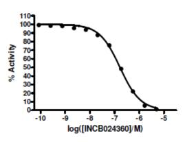
IDO1 activity (right) and IDO1 inhibition (left), measured using the IDO1 protocol for the Universal Inhibitor Screening Assay Kit, BPS Bioscience, Catalog #72035. Data shown is lot-specific. For lot-specific information, please contact BPS Bioscience, Inc. at info@bpsbioscience.com.
