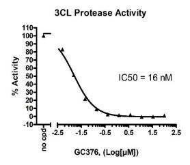
Inhibition of 3CL Protease enzyme activity by GC376, measured using the *Untagged 3CL Protease (SARS-CoV-2) Assay Kit (BPS Bioscience #78042)*. Fluorescence intensity was measured using a Tecan fluorescent microplate reader. *Data shown is lot-specific*.
