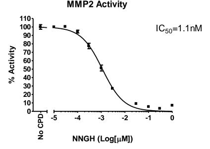
Inhibition of MMP2 enzyme activity by NNGH, measured using the *Fluorogenic MMP2 Assay Kit (BPS Bioscience #79918).* Fluorescence intensity was measured using a Tecan fluorescent microplate reader. *Data shown is lot-specific. For lot-specific information, please contact BPS Bioscience, Inc. at <u>info@bpsbioscience.com</u>*
