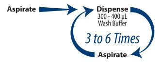
2. Ensure that the plate washer has a program that will not scratch the bottom of the microplate and will prevent plate drying. This is critical to prevent damage to the capture antibody arrays. The simplest method to avoid plate drying is to leave a small, uniform amount (1-3  $\mu$ L) of wash in the well after the final aspiration, and add the next reagent to the plate as quickly as possible.
