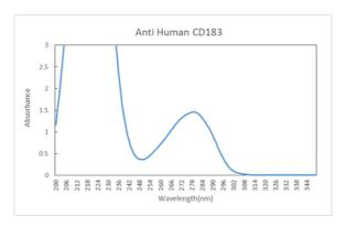
Description: 1 mg/mL Mouse anti human CD183, the protein type was Mouse IgG1, PBS (pH 7.2, no preservatives), measured by the Nano 100 spectrophotometer, the concentration curve was normal, and A280=1.454, in line with the labeled concentration.
