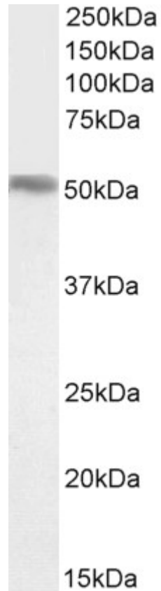
EB05999 (0.1 \mu g/ml) staining of Mouse Liver lysate (35 \mu g protein in RIPA buffer). Detected by chemiluminescence.
