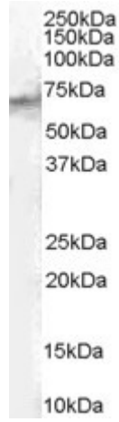
EB07213 (1 \mu g/ml) staining of Human Spleen lysate (35 \mu g protein in RIPA buffer). Detected by chemiluminescence.
