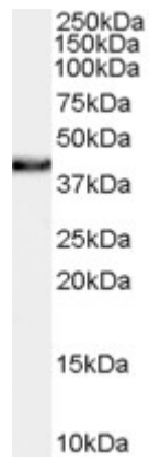
EB07440 (0.1 \mu g/ml) staining of Human Thyroid lysate (35 \mu g protein in RIPA buffer). Primary incubation was 1 hour. Detected by chemiluminescence.
