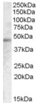
EB08189 (0.1 \mu g/ml) staining of A431 cell lysate (35 \mu g protein in RIPA buffer). Primary incubation was 1 hour. Detected by chemiluminescence.
