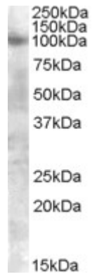
EB08456 (0.3 \mu g/ml) staining of A549 lysate (35 \mu g protein in RIPA buffer). Primary incubation was 1 hour. Detected by chemiluminescence.
