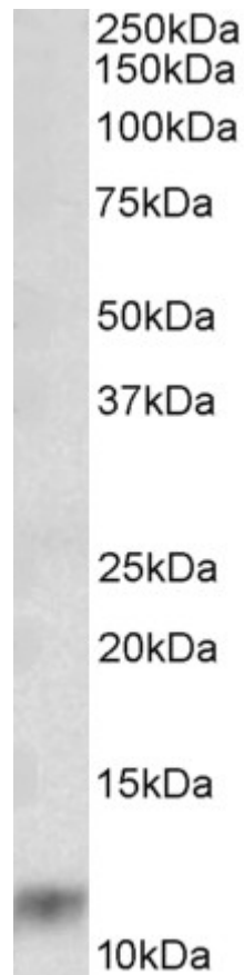
EB11513 (0.03 \mu g/ml) staining of Human Lung lysate (35 \mu g protein in RIPA buffer). Detected by chemiluminescence.
