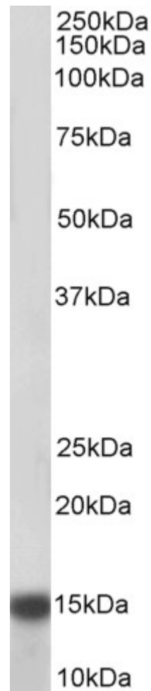
EB11683 (0.1µg/ml) staining of Pig Heart lysate (35µg protein in RIPA buffer). Detected by chemiluminescence.
