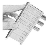
Figure 3: Hand-decanting supernatant using a Magnetic Rack.
