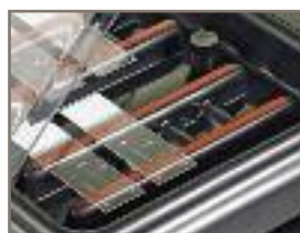
Wells between rails can be used to hold water for techniques needing a humid environment.
