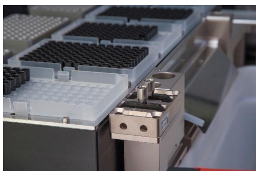
CO-RE Gripper holder with jaws for the 1000 µl pipetting channels (inner positions)
