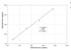
Linearity was determined by taking two human urine samples diluted 1:140, one with a low diluted cortisol level of 163.9 pg/mL and one with a higher diluted level of 2,974.9 pg/mL and mixing them in the ratios given below. The measured concentrations were compared to the expected values based on the ratios used.
