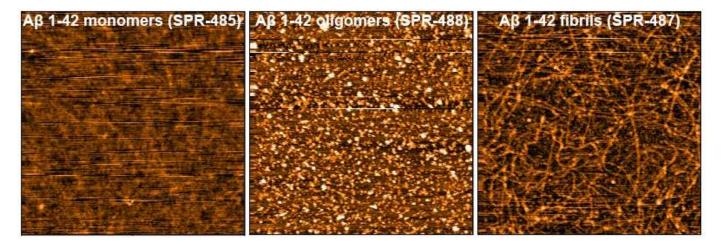
AFM of amyloid beta 1-42 monomers (SPR-485, left), oligomers (SPR-488, middle) and fibrils (SPR-487, right). Atomic force microscopy analysis of 1.0 mg/mL samples diluted to 0.1 mg/mL in dH2O, mounted on freshly cleaved mica, washed, dried and analyzed with tapping mode. Representative images are  $2.5 \times 2.5 \, \mu m \, x$ -y with a z-range of 10 nm.
