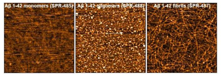
AFM of amyloid beta 1-42 monomers (SPR-485, left), oligomers (SPR-488, middle) and fibrils (SPR-487, right). Atomic force microscopy analysis of 1.0 mg/mL samples diluted to 0.1 mg/mL in dH2O, mounted on freshly cleaved mica, washed, dried and analyzed with tapping mode. Representative images are 2.5 x 2.5  $\mu$ m x-y with a z-range of 10 nm.
