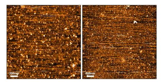
Atomic force microscopy analysis of 2 mg/mL SPR-497 diluted to 0.2 mg/mL with dH2O mounted on freshly cleaved mica, washed, dried and analyzed with tapping mode. Representative images are 2 x 2  $\mu$ m x-y (left) and 5 x 5  $\mu$ m x-y (right), both with a Z-range set at 4nm.
