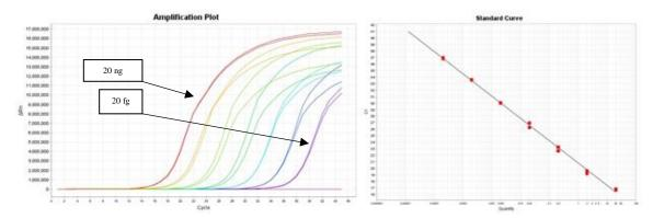
Reliable standards for the quantification of fungal DNA: Fungal DNA Standards (measured in duplicates) comprise 10-fold dilution series ranging from 2 ng to 20 fg.
