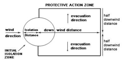
From IERG (Canada/Australia) Isolation Distance -Downwind Protection Distance -
